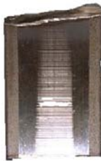
Figure 1: Section of outer race of AC variable speed motor roller bearing showing fluting
