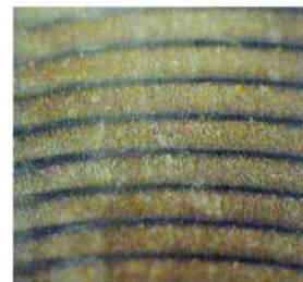
Figure 2: Section of inner race of DC motor ball bearing showing fluting
